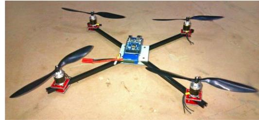
Fig.10 Manufactured chassis
