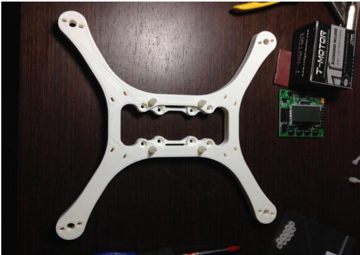
The frame with the nylon supports for the control board fitted.
