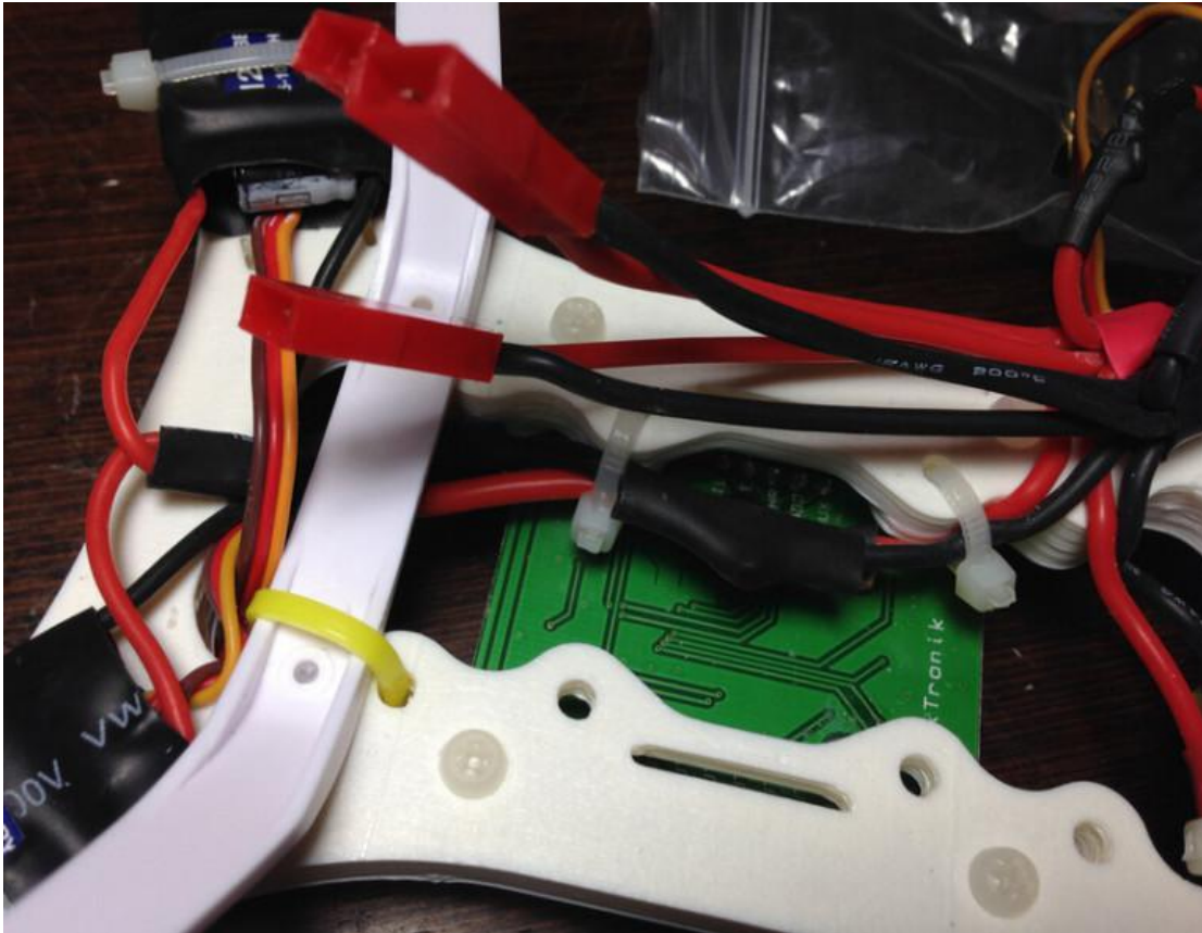
Wiring of the ESCs, detail
