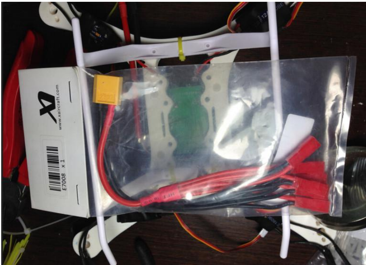
Landing gear glued and zip-tied in place
